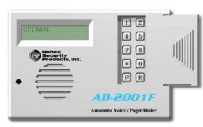
The AD-2001F dialer features busy-line and no-answer detection to ensure prompt transmission of up to 2 prerecorded messages delivered sequentially to as many as 4 standard telephones, cellular phones, voice and/or numeric pagers. Messages to both local and long-distance calls can be transmitted. When activated, the dialer instantly begins calling the numbers in sequence, delivering each message 1 to 3 times in a row, in accordance with the preselected number of dialing attempts.
